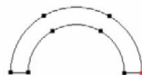
Figure 6-41 The closed spline after using the Outline button on the open spline
